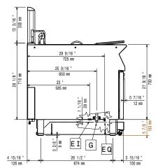
ΕI Electrical inlet (power) EQ Equipolential screw Gas connection
